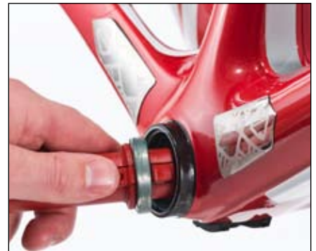
Figure 23. Pressing the bearing into the frame
